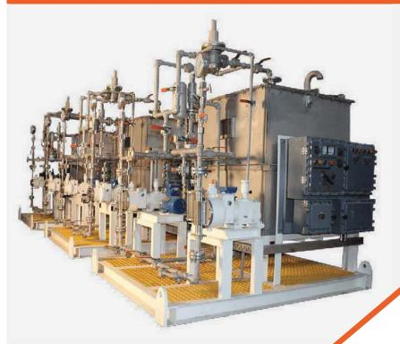
**Additive Injection Package For Jet** Fuel System -**Supplied to Europe**
